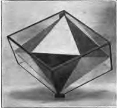
FIG. 86.—Rhombohedron ( R ) resulting from disappearance of darkened planes of the interior figure—a hexagonal bipyramid.
